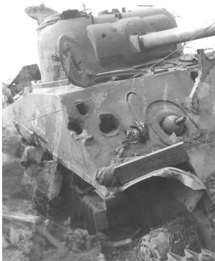
Apparent exit holes in the glacis of a knocked out Sherman – 1945
