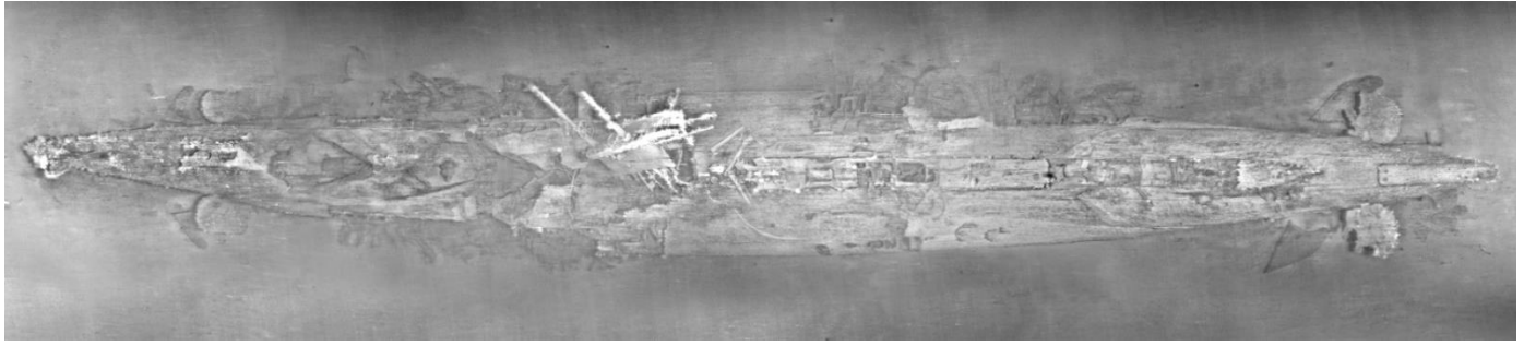
A detailed two-dimensional photomosaic of AE1 was generated from over 6,000 digital images taken by Fugro Equator's AUV
