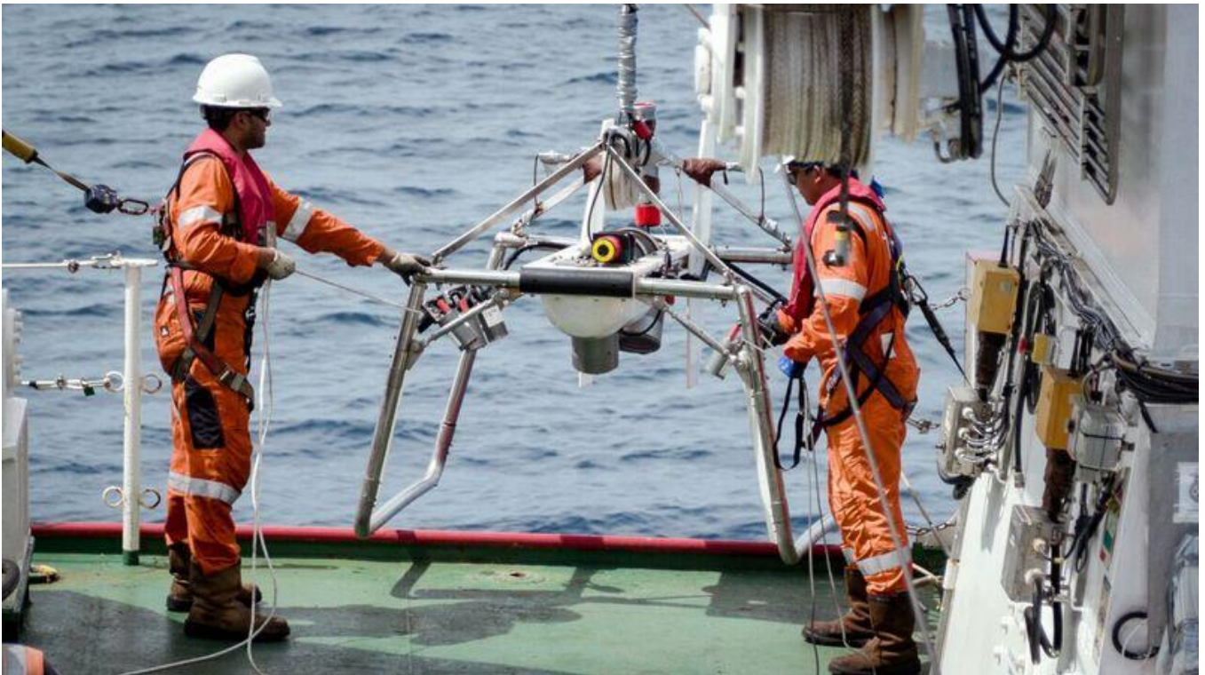
A drop-camera was used to examine the side scan sonar 'contact of interest' that was ultimately identified as AE1
