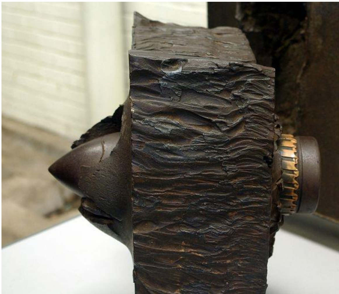
Armor piercing shell from a 17-pdr gun embedded in a section of armour from a Tiger I tank
