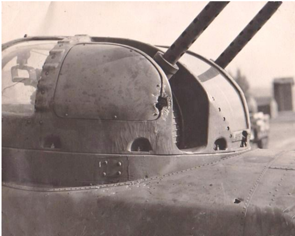
"A 20mm cannon shell entered the top turret, hit the armor plate on back of my seat and exploded, knocking out the left side window and puncturing my eardrum, showering plexi-glass all over. Only me and the laundress know how close this one came"
