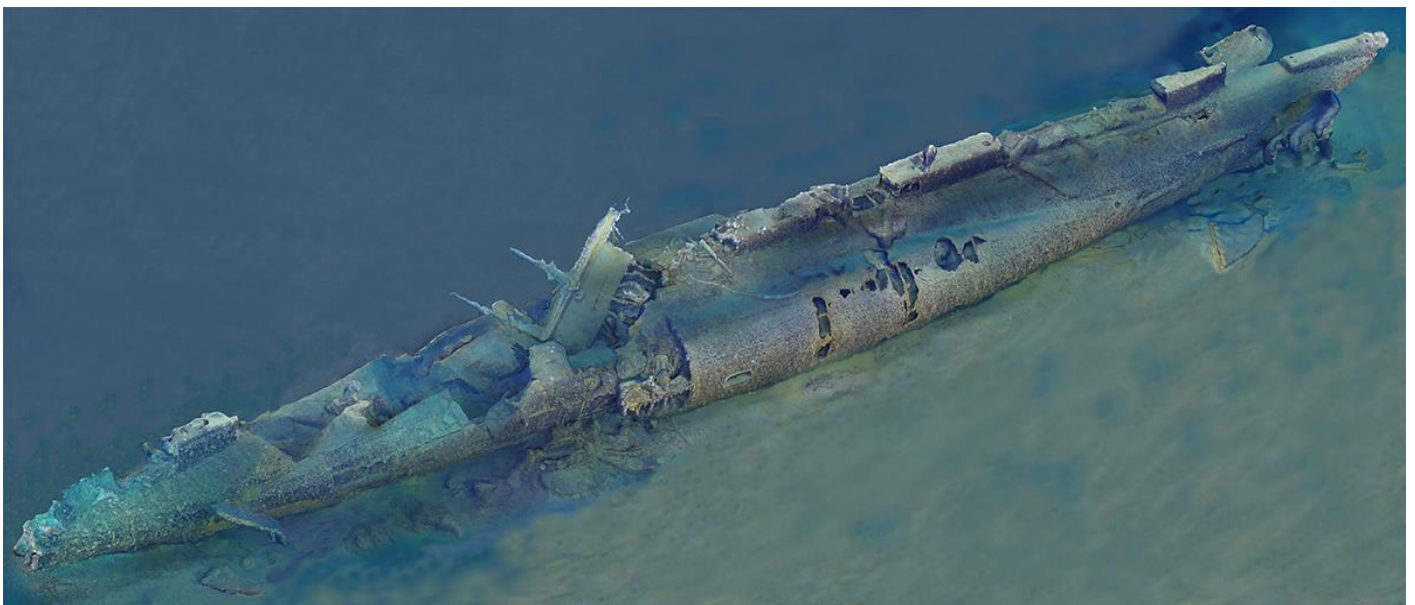
Port side view of the interim 3D photogrammetric model of AE1. A high-resolution 3D model is currently being generated from the more than 8,000 still images at Curtin University's HIVE (Hub for Immersive Visualisation and eResearch)
