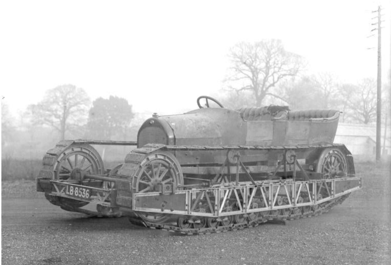
Experimental Light "D" Tank. Experimental tracks fitted to Overland Chassis
