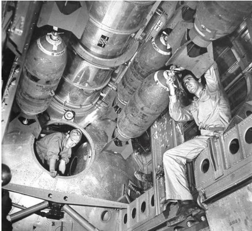
Personnel inserting fuse into a 500 lb. demolition bomb in the bomb bay of B-29 Superfortress, China, June 1944
