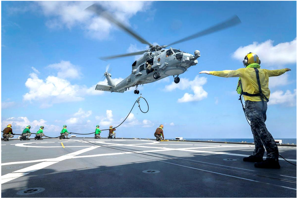
HMAS Stuart conducted a Helicopter in-Flight Refuelling (HIFR) evolution from the flight deck, with their embarked Flight 602 MH-60R Seahawk helicopter call sign 'Scarecrow' during the ship's regional presence deployment
