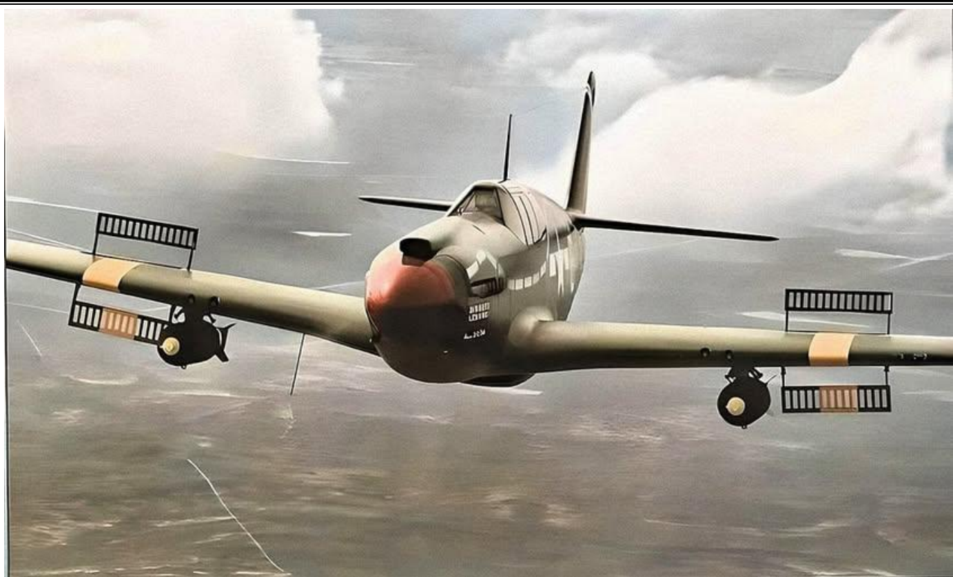
A-36 Mustang with diving brakes engaged
