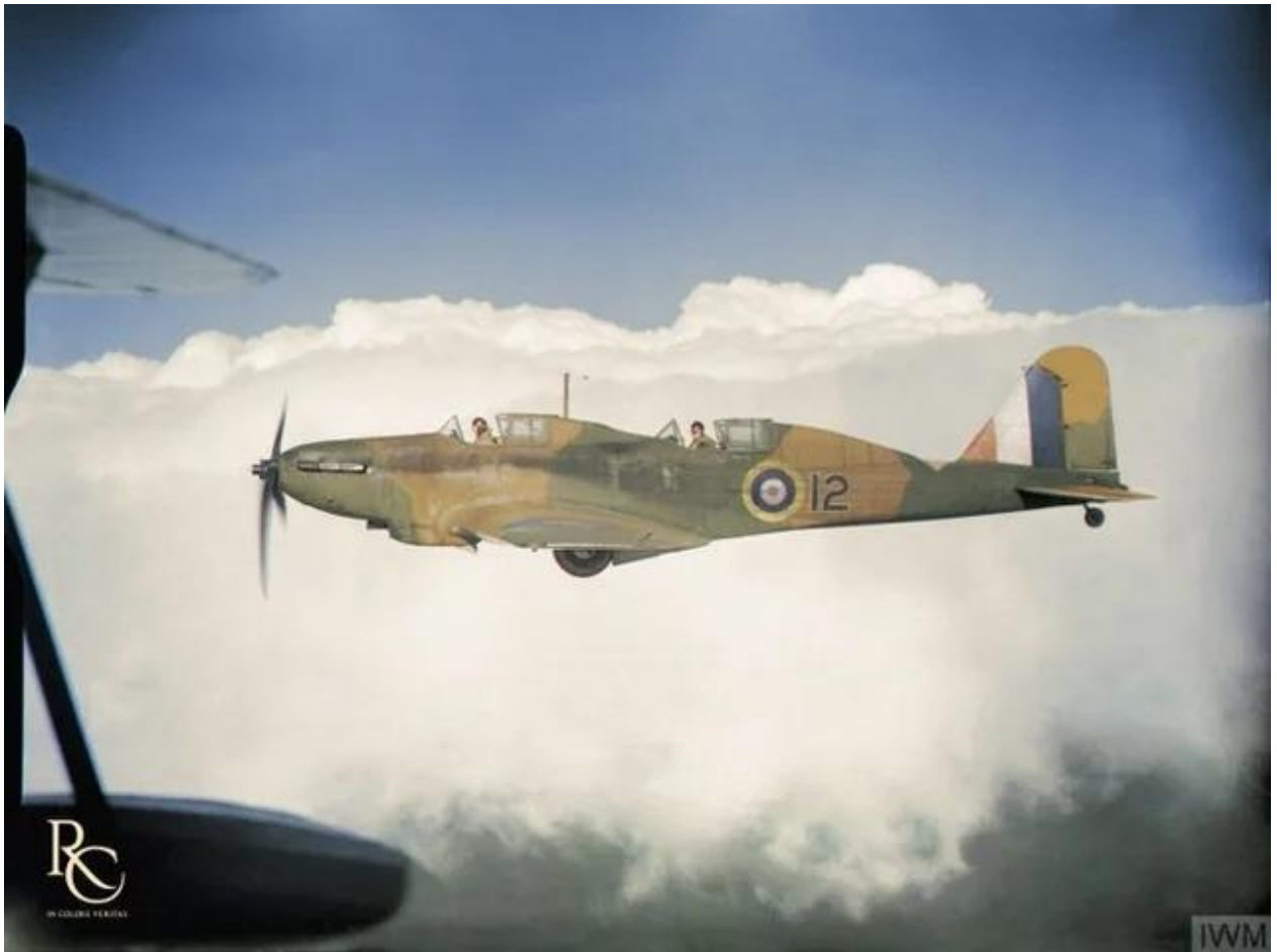
There are some visually unpleasant aircraft in WW2, but the Fairey Battle conversions into trainers with 2 cockpits stand out
