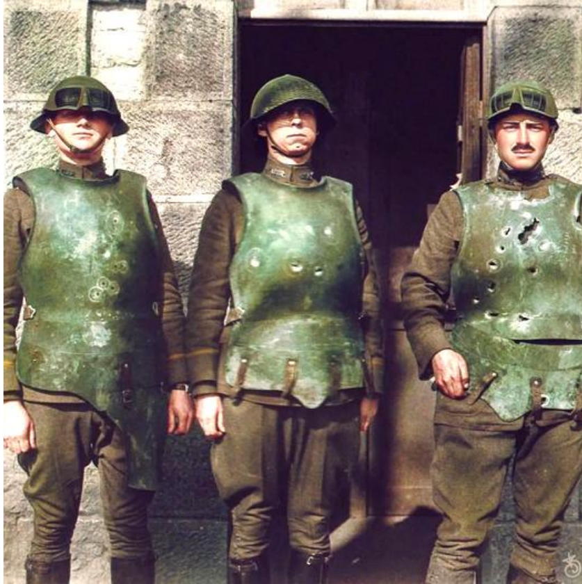
U.S. soldiers wearing experimental body-armor and helmets displaying results of bullet testing, April 27, 1918.
