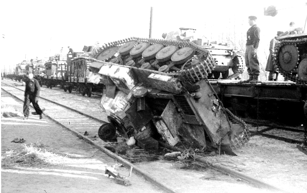
A Pz.Kpfw II after falling from a railway platform during loading, May 1943
