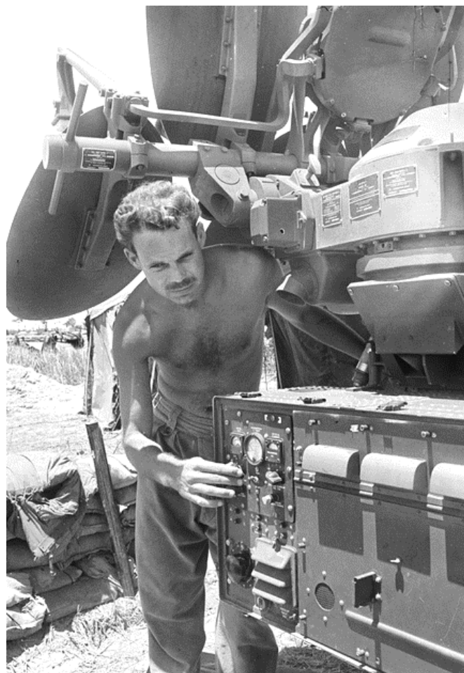
Bombardier Keith Hylife, 131st Divisional Locating Battery, checks radar equipment used to pinpoint enemy mortars being used in attacks on Coral
