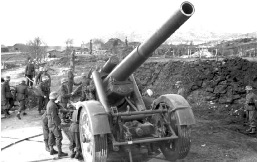
The German 21 cm Mörser 18 heavy howitzer at Bodø, Norway, in fall 1943, was known for its dual-recoil system and two-part transport for easy deployment.
