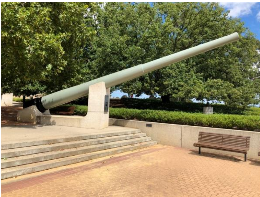
Left: One of HMAS Australia 's 8-inch gun barrels on display in the grounds of the Australian War Memorial Canberra. Right: A similar barrel as fitted to the ship when in commission. Each barrel weighed 17.3 tonnes and could fire a 116kg projectile 26.7kms. The life of each barrel was 550 rounds.
