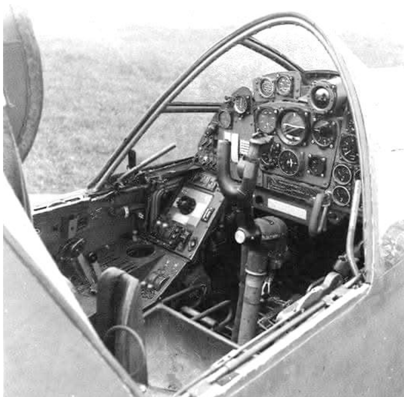
A great photograph of a Dornier Do 335 cockpit. This aircraft was fitted with an ejection seat powered by compressed air... In addition, explosive bolts blew off the rear propeller and tail fin so the pilot wouldn't impact them upon leaving the aircraft
