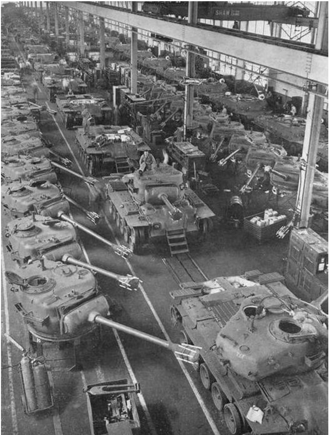
The M26 Pershing assembly line at the General Motors Grand Blanc tank plant in Michigan, 1945.
