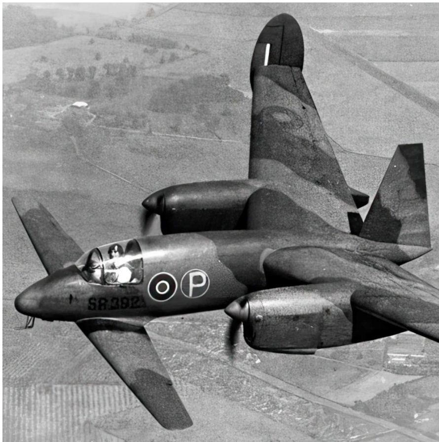
The Miles M.39B Libellula, a distinctive twin-fuselage, tandem-wing aircraft, originated in the heart of World War II. The brainchild of British aviation engineer and designer Frederick George Miles
