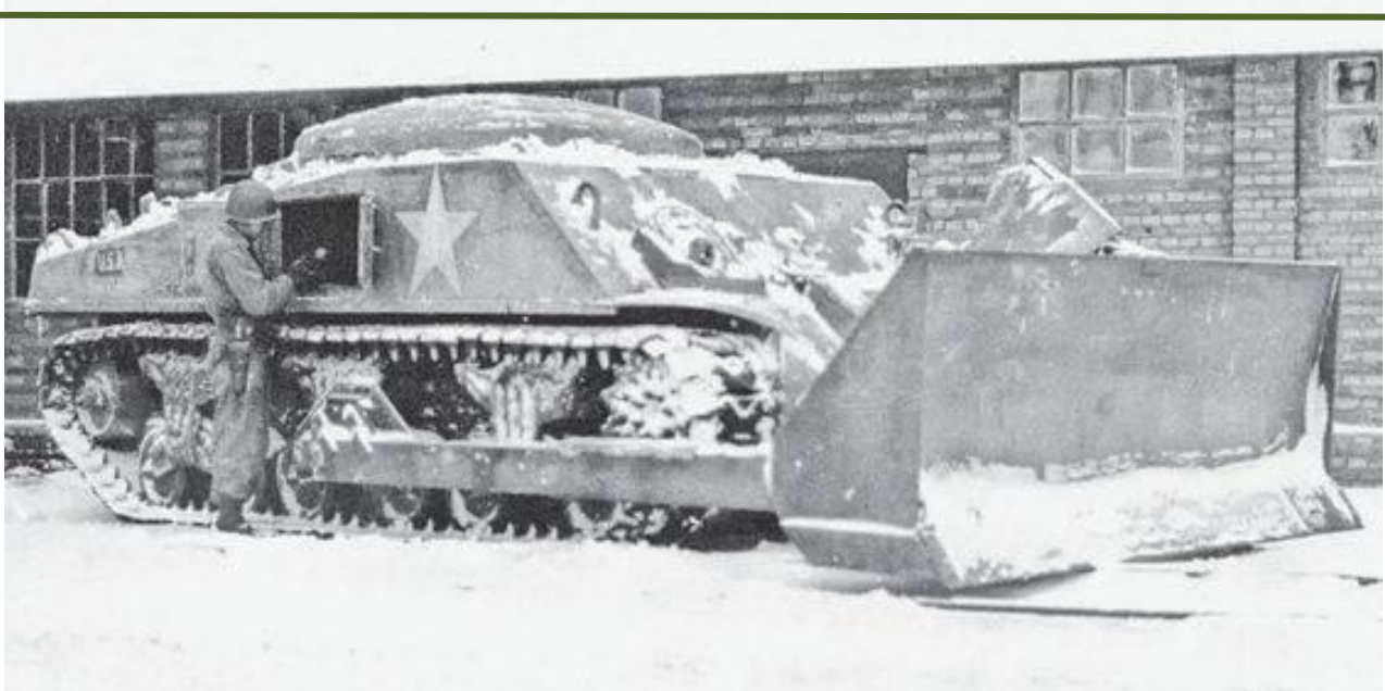
M4A3 Sherman converted into a bulldozer.
