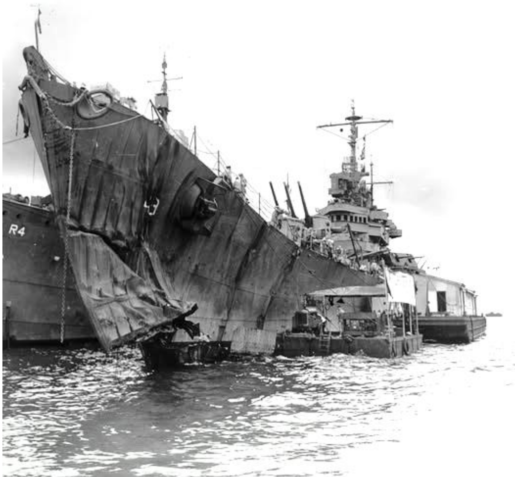
Cruiser USS St. Louis with visible torpedo damage from the Battle of Kolombangara, Espiritu Santo, July 1943
