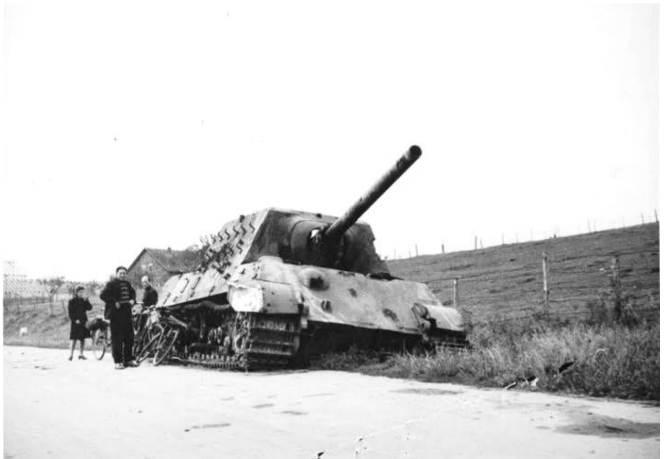
A German Jagdtiger (Panzerjäger Tiger Ausf. B, Sd.Kfz. 186) of the 512th Heavy Tank Destroyer Battalion lies destroyed on a road near Osterode. The massive vehicle is missing its left armour plate, the roof of the fighting compartment, and the gun mantlet, damage consistent with having been blown up by its own crew.
